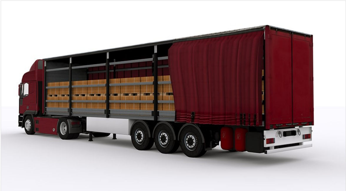
Curtainsider loaded with pallets. Source: Topai/Shutterstock.com
