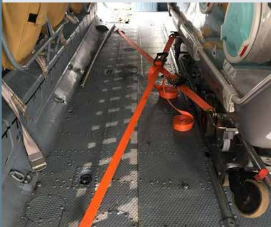
An individual isolation unit is safely fixated to the frame of an airplane for HID transport. Norway, 2020. ©Norwegian Directorate of Health
