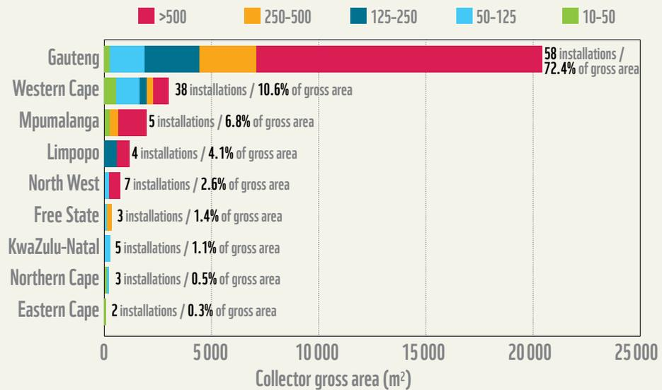
As can be seen in Figure 11, most large-scale solar thermal systems are in Gauteng, with 58 installations in total, accounting for 72,4% of the gross collector area installed throughout South Africa. Figure 12 shows the gross collector areas for the various applications that have solar thermal systems installed. The different applications for which the database is categorised include process heat, cooling and domestic purposes, which include hot water for staff ablutions in buildings.
