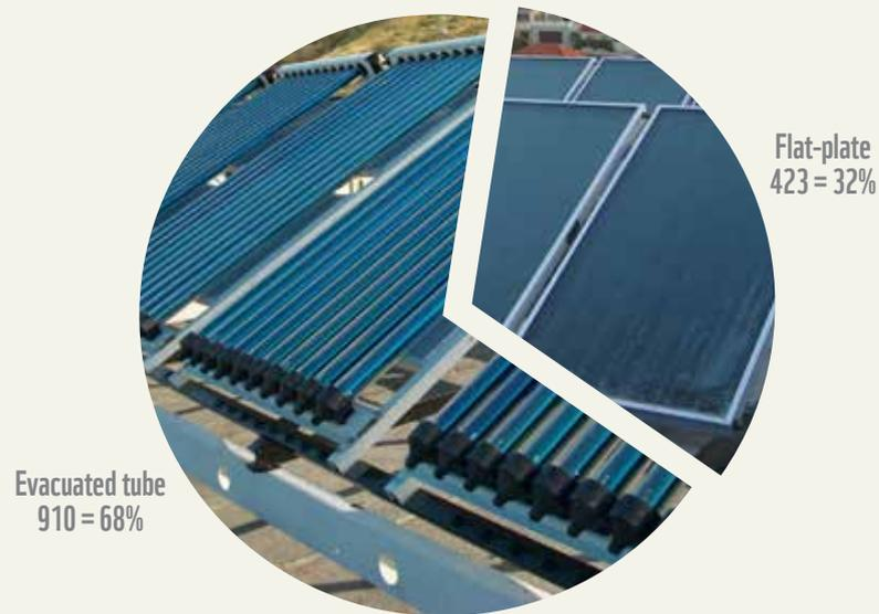
Figure 24 shows that evacuated tube collectors are the most commonly installed solar technology to supply the 60 °C hot water temperature requirement of hospitals, accounting for 910 m<sup>2</sup> (68%) of the 1 333 m<sup>2</sup> of total collector area installed at hospitals in the country.
