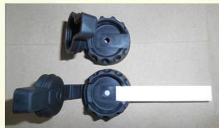
2. Lift the flap on the head of the black cap and slide a test strip into the groove so that the reaction zone faces the small opening and completely covers it. Secure by pressing the flap back in place.
