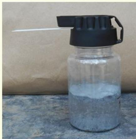
11. Remove the Test Strip after 20 minutes from the black cap and match colour with the '50ml, 0-500' serial colour chart. The colour of the Reaction zone of the test strip will indicate the level of arsenic present in the sample water.
