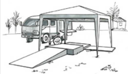
Blocks and 1:12 ramp
