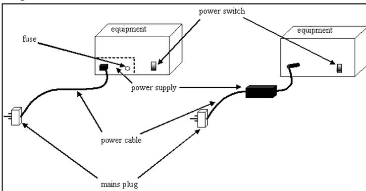
General item of electrical equipment, one with internal power supply, the other with external
