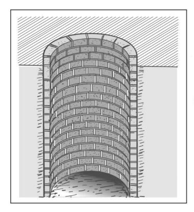
The whole pit will be lined with concrete bricks or rubble stones. You will need 24 bricks for the top 50 cm (and the above ground level part), and 33 bricks for each meter of the rest of the pit.
