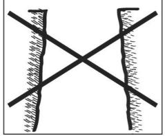
The diameter of the pit must be uniform throughout and the walls must be vertical.
