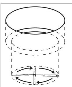
To avoid this kind of situation a simple tool can be used every 50 cm when deepening the pit to assure that an even diameter of the pit is maintained. This simple tool can easily be made of two pieces of wood, each wood to be exactly as long as the diameter of the hole and fastened at 90° at the centre.
