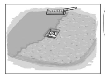
To complete this slab, an impermeable and smooth surface is added onto the top with lateritic soil mixed with animal dung (cow dung) or with a decoction of Nere tree seed pods. Some people use simple termite-hill soil.
