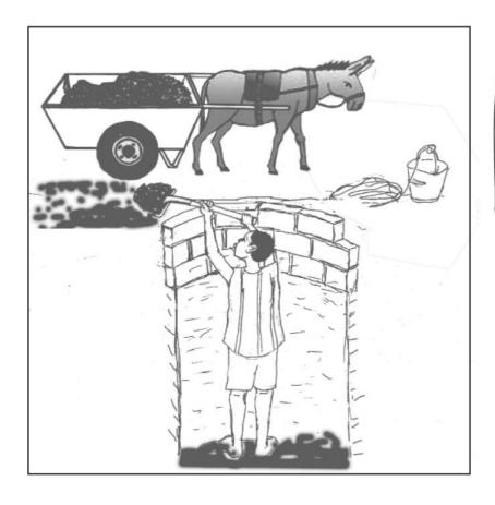
When the second pit is full, the faeces of the first pit will be well decomposed and safe and can be used as a natural fertilizer, and then after emptying it you can reuse the pit as a latrine again.
