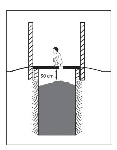
The second pit must be dug when the faeces in the first pit reaches to 50 cm below the ground level. The second pit must be located at least 3 m from the first one.
