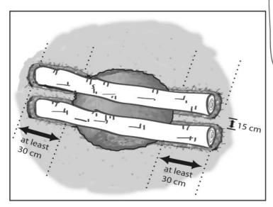
You must use 2 big logs about 15 cm apart, that can support the weight of the slab plus the weight of the user. If the pit is not lined, these logs must be long enough to rest on the soil well beyond the limit of the pit, 30 cm at least. A hard wood must be used. This wood must not rot, or be easily attacked by termites.
