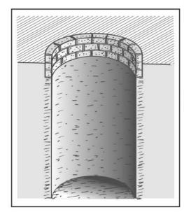
In an area where the soil is stable, it is not necessary to line the whole pit. Only the top 50 cm will be lined.
