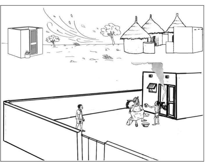
The latrine must not be located in a place that can flood.
