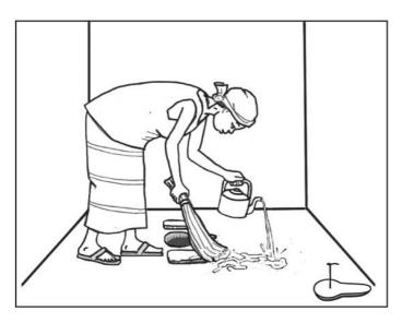
The slab must be cleaned regularly.
