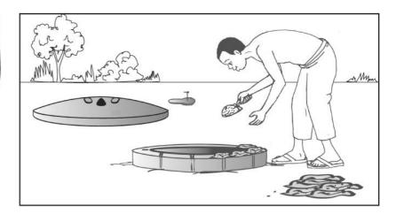
The slab must be well centred and well seated on the sub foundation.
