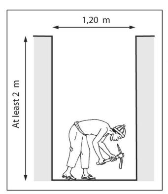
If the soil is unstable, the diameter of the pit must be uniform throughout its entire depth and will be of the same diameter as the slab (1.20m)
