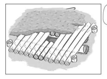
After this, you must compact a layer of soil on the wood. It is important to use a good soil for the compacting, a lateritic soil for example.
