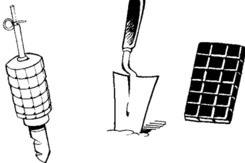
The surface thus looks very much like a bar of chocolate divided into squares. When it explodes, the casing breaks at the weakest point – along the criss-cross of grooves – and razor-sharp squares of metal fly in all directions.
