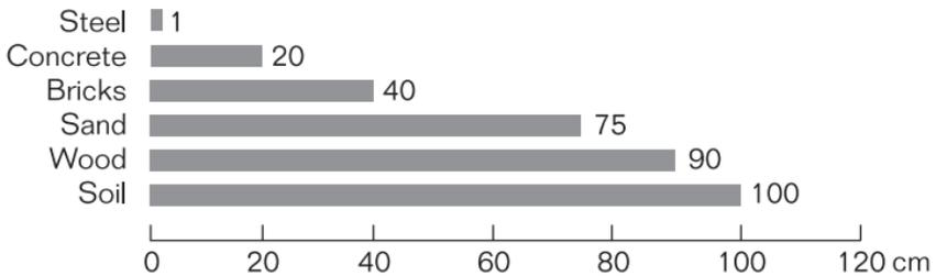
Note that these thicknesses are good only against sporadic fire. Protection against continuous firing would require double the thicknesses indicated.
