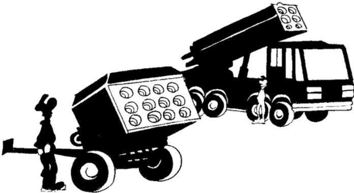
**Anti-aircraft guns.** These are mentioned because, though designed to shoot down aircraft, they can also be used against targets on the ground. Owing to the excellent sights and accuracy of these weapons, they pose a very dangerous threat. Generally they are light and portable. Some have multiple barrels. Their range is from 2 km for the smaller versions and up to 8.5 km for the larger, towed guns. The rounds used are from 20 mm to 40 mm in calibre.
