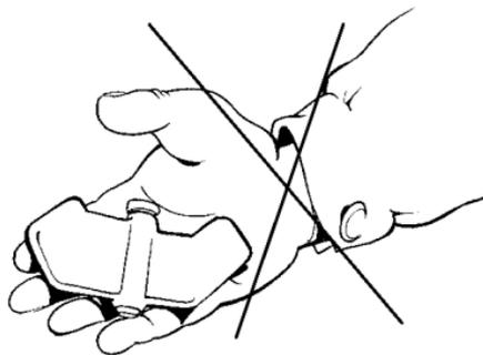
such seeds spiralling down from a tree in the autumn; they catch the wind and spread out over a wide area. The butterfly mine is shaped in a very similar way and with the same intent. It is dropped from the air and gently spirals down to earth. Thousands are dropped at a time and spread out over a large area. Normally blue/
