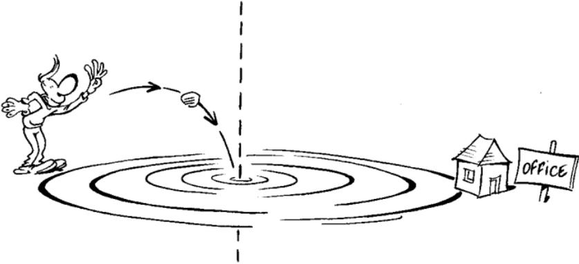
You see that the waves are travelling in a plane horizontal to the antenna. If it is sloping backwards, you are sending excellent signals to Mars, perhaps, but not to your office!
